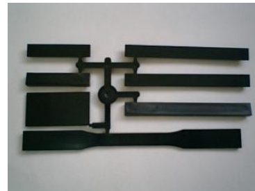
(Test Pieces for Various Physical Properties Test )
